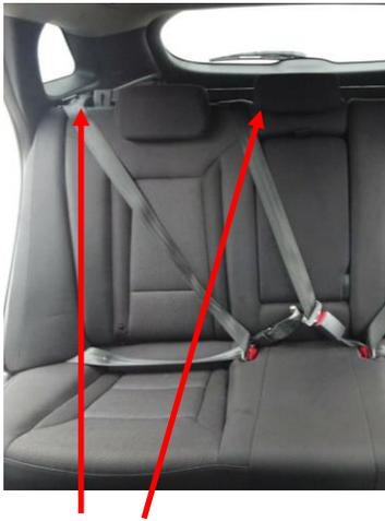
The retractor is attached to the vehicle frame within the seat structure at the end of the shoulder belt.
