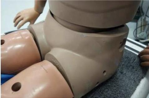
The dummies are designed this way to increase the likelihood that the dummy will always be placed in a similar way. The downside of this good repeatability is that the pelvis will not behave like a human pelvis and cannot be used to detect possible injury to the major blood vessels that are present in this region in a human (i.e., femoral arteries).
